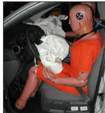
These kind of test are common for many companies but represent a high inversion for them. The crash-test dummies used are rubber-skinned, with steel 'skeletons', and each one costs around £100,000 on account of the sensors they incorporate to provide the data.
