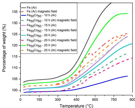
**Figure 6.** Variation of weight as a function of temperature for the sample of pure Fe, Fe<sub>50</sub>Co<sub>50</sub> at different milling times under argon atmospheres in the absence and in the presence of an external magnetic field, in the temperature range between 25 °C to 900 °C.
