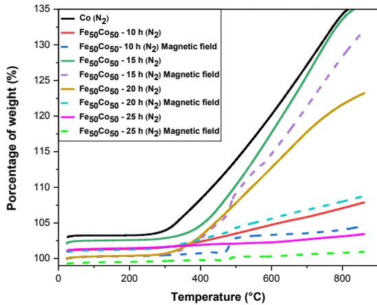
**Figure 7.** Variation of weight as a function of temperature for the sample of pure Co,  $Fe_{50}Co_{50}$  at different milling times under nitrogen atmospheres in the absence and in the presence of an external magnetic field, in the temperature range between 25 °C to 900 °C.
