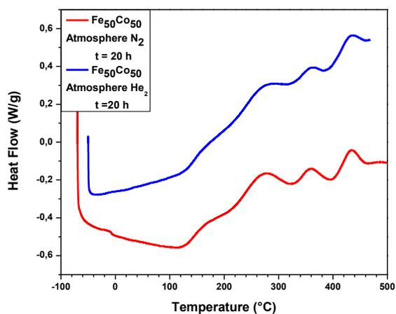
**Figure 4.** DSC curves for the Fe<sub>50</sub>Co<sub>50</sub> sample milled 20 hours under N<sub>2</sub> and He atmosphere in the temperature range between -60 °C to 500 °C.
