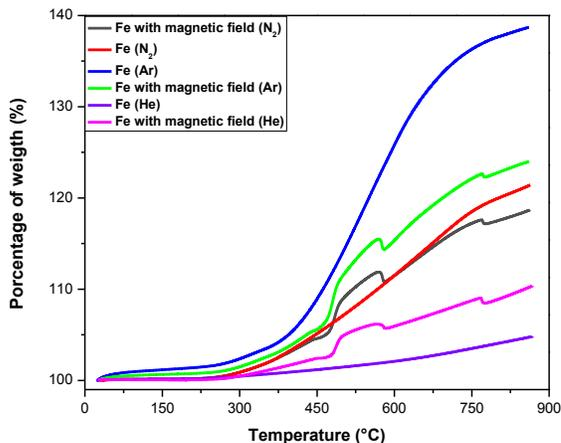
**Figure 5.** Variation of weight as a function of temperature for the Fe sample under atmospheres of nitrogen, helium and argon in the absence and in the presence of an external magnetic field, in the temperature range between 25 °C to 900 °C.
