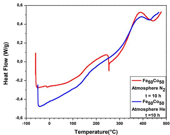
**Figure 3.** DSC curves of the Fe<sub>50</sub>Co<sub>50</sub> sample milled 10 hours, under N<sub>2</sub> and He atmosphere in the temperature range between -60 °C to 500 °C.
