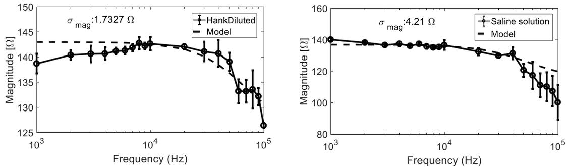
**Figure 5.** Spectra of the magnitude of the impedance for Hanks' and deionized water solutions with dilute sodium chloride.
