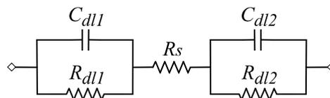
**Figure 4.** The proposed EEM for polar solution IS measurements using the reusable wells.
