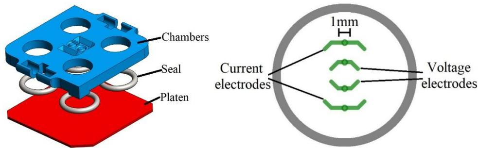
**Figure 1.** Reusable 3D-Printed wells. (a) Exploded view of the device with four wells for IS measurements of aqueous solutions and (b) top view of the electrode array of one well.
