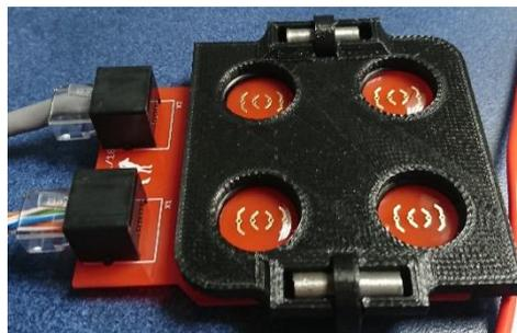
**Figure 2.** Four 3D-printed reusable wells, each one with 1 ml of an aqueous solution.
