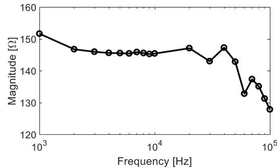
**Figure 3.** Bode plots for Hanks' solution (buffer solution).
